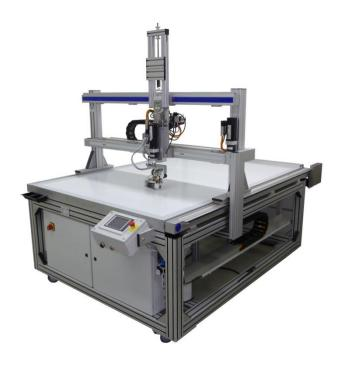
The PVB sheets are placed on the table and held by vacuum. A busbar laying head holds the busbar spool, busbar guidances and a heating roller. The head performs movement with two linear and one rotary axes. It is fully CNC programmable and therefore not constrained to any busbar geometry.
